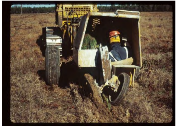
Machine planting pine seedlings. (note: the green side is up, nearly straight with the roots below the ground line, minimal soil disturbance)
